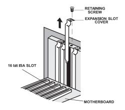
Figure 2: Removing the Backplate
